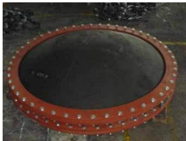
It is normally pierced by a pile with an Inflatable Grout Packer, and often used together with either an Inflatable Grout Packer or Grout Seal and Mud Wiper to ensure that no seabed materials ever enter the sleeve.
