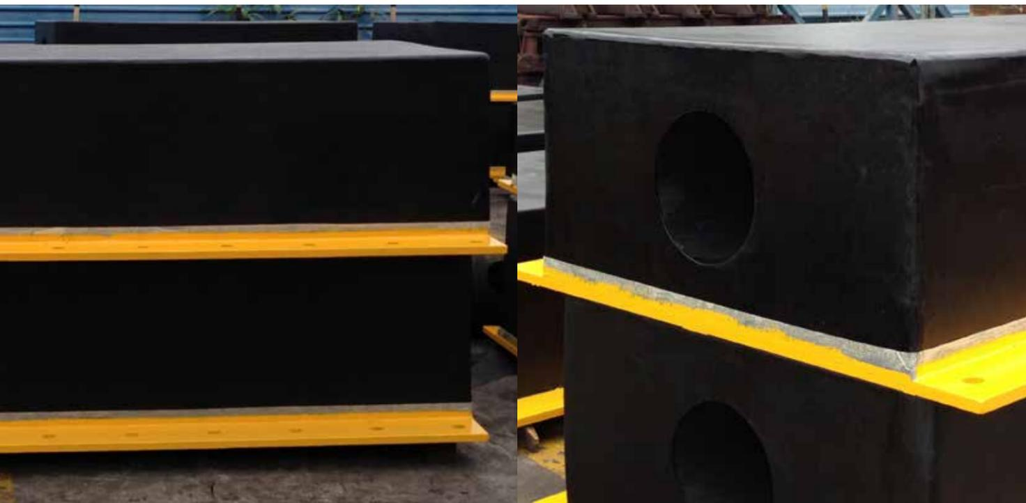
Barge fendering systems are used during the float-over operation, and protect against damage arising from potential impact between the barge and the substructure legs during the entrance, mating and exit phases. The fenders also assist in ensuring the design clearances during this operation.
